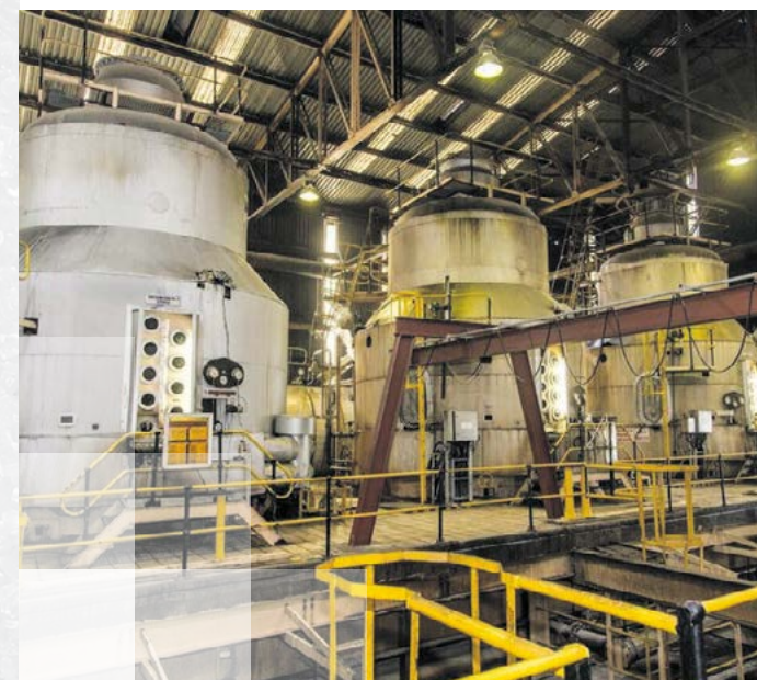
Vacuum pans inside the Royal Eswatini Sugar Corporation Simunye Mill
